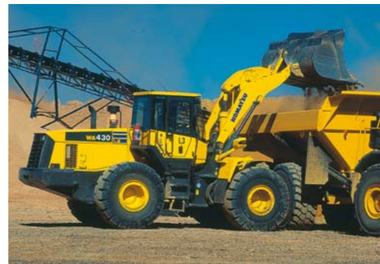
One of the Komatsu WA430-5 wheel loaders loading an ADT at Wouterspan.
