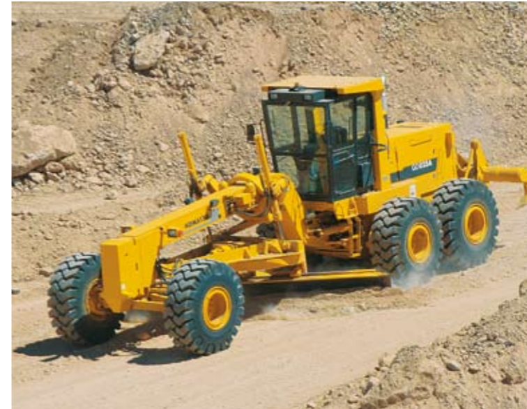
The Komatsu GD825A- 2 articulated motor grader busy with haul road maintenance.
