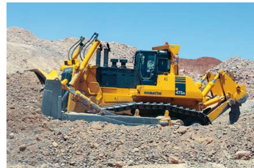
One of the Komatsu D475A-5 crawler dozers stock piling alluvial gravel for a PC800SE-7 hydraulic excavator to load.
