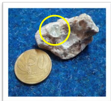
Diamond locked up in calcrete that would be lost without proper liberation
